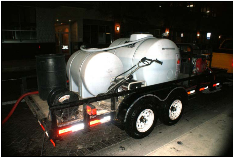
Figure 12. River Walk Implementation Plan power washer which recaptures the wastewater.
