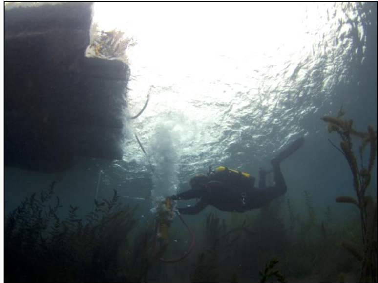
Figure 16. Core tube being driven using pneumatic post driver.
