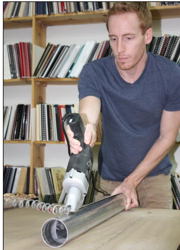
Figure 18. Author using electric tin shears to cut aluminum core tube.
